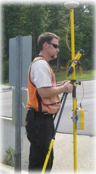
Greene Surveying in Marion, is operating his \$35,000 GPS gear to set one of two GPS benchmark points for the bottom mapping team to use as references. These known control points will be utilized as checks at the start and finish of each mapping run. If lake elevation and GSP coordinate readings at the benchmarks disagree significantly with those from Duke Energy's posted lake elevation or our equipment readings of
